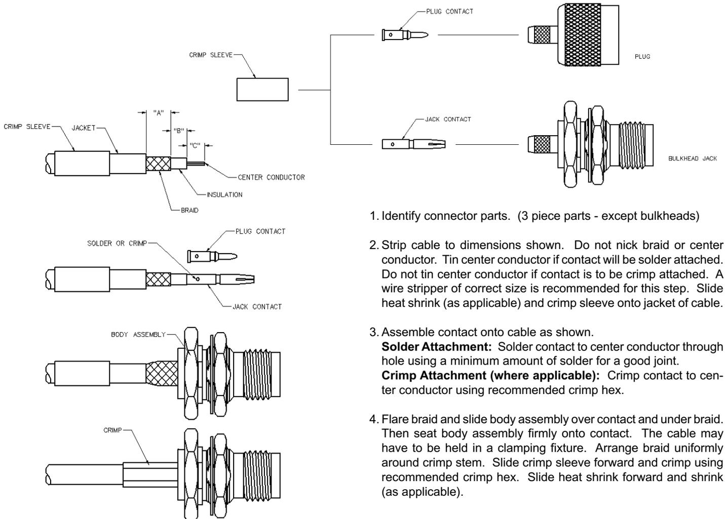
1. Identify connector parts. (3 piece parts - except bulkheads)
